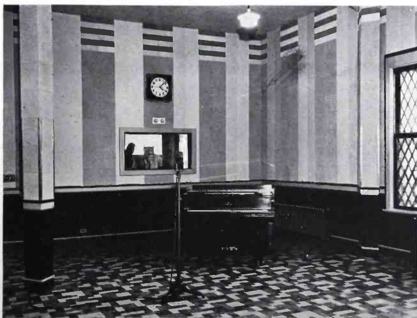
THROUGH THE TRIPLE-PLATE GLASS SOUND-PROOF WINDOW IS THE ORGANIST'S ROOM, WHERE THE PROGRAM MAY BE HEARD ONLY THROUGH A MONITOR LOUDSPEAKER. THERE THE MONITOR OPERATOR (WITH HIS CONTROL EQUIPMENT) IS ALSO LOCATED, CLOSE TO THE ORGAN CONSOLE
