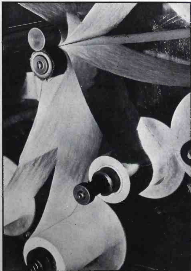
FARADON CONDENSERS IN THE MAKING, AT "RADIO HEADQUARTERS," CAMDEN, N. J.
